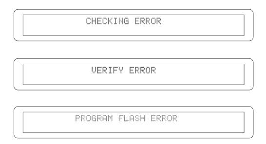
A serious error has occurred during loading of the firmware into the memory. Contact your nearest service centre, stating the type of error shown on the display.
